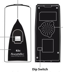
To set the device ID of the terminal. Use this only if you are installing the terminal with an Ingressus controller.
